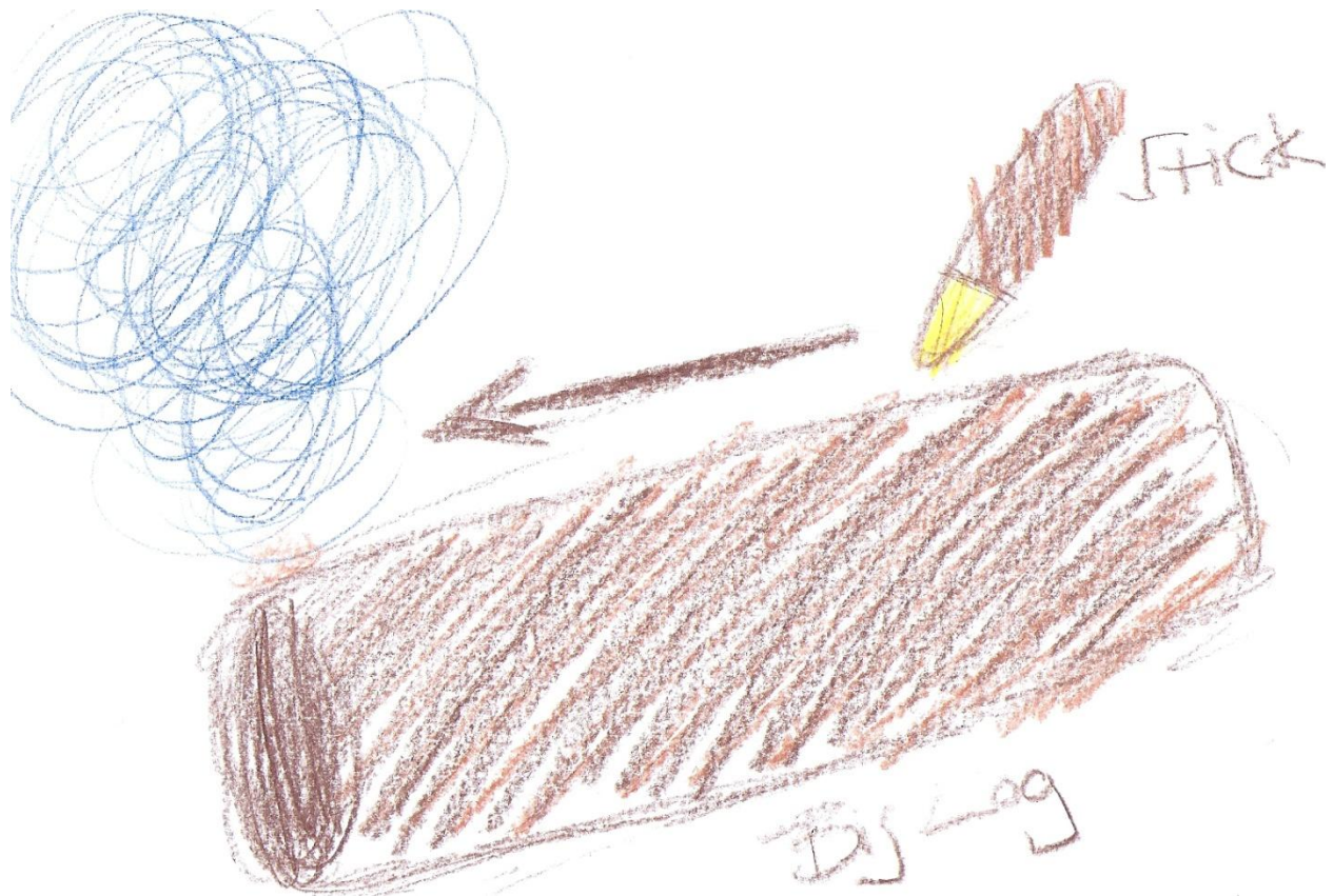
Image #4 – Group 1, initial heat energy design. This design is based off of the “fire plough” method of rubbing a small stick on a larger log to generate a coal. One student from the group mentioned that he had seen his uncle start a fire in this fashion which ultimately led the group to go in that specific design direction
